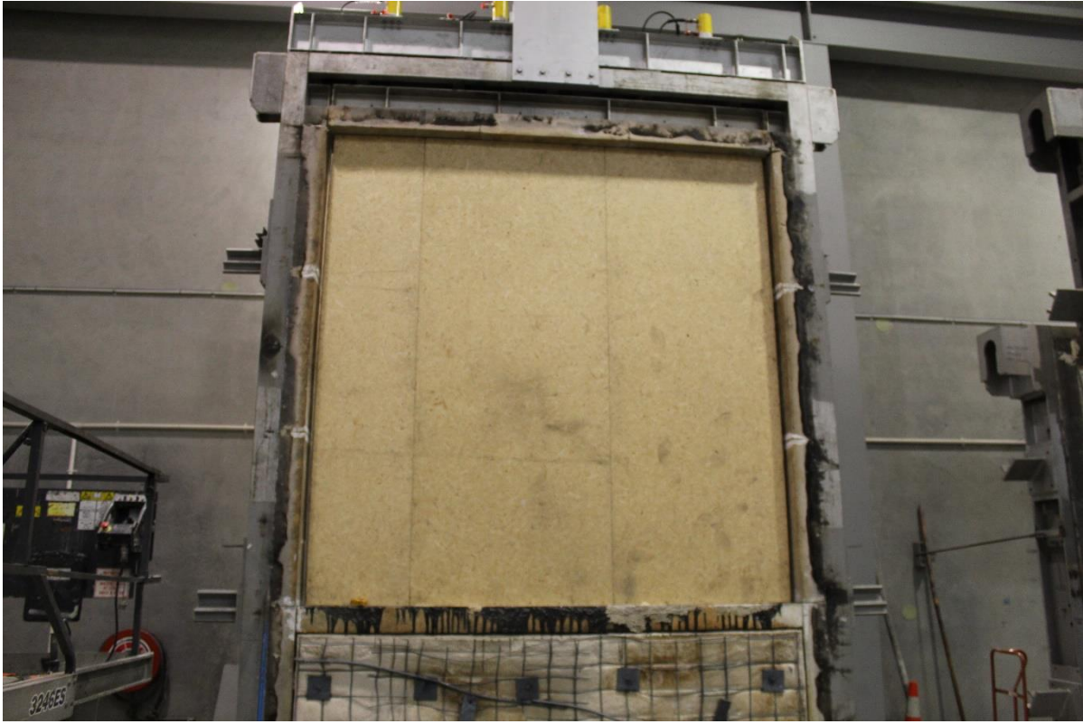
Exposed face after plasterboard lining:
