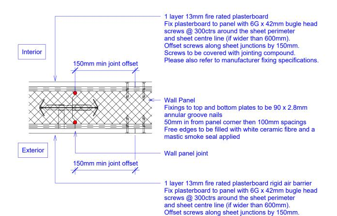
Screws to be covered with weathertight sealing tape. Please also refer to manufacturer fixing specifications.
