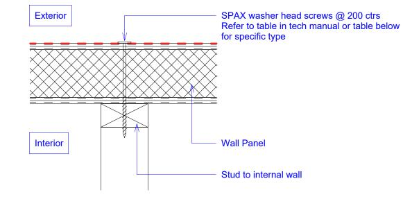
Washer Head type screws for fixing roof panels, wall panels and beams together are selected from the following.
