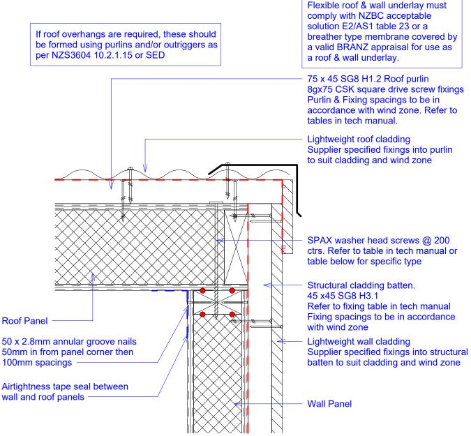
Washer Head type screws for fixing roof panels, wall panels and beams together are selected from the following.
