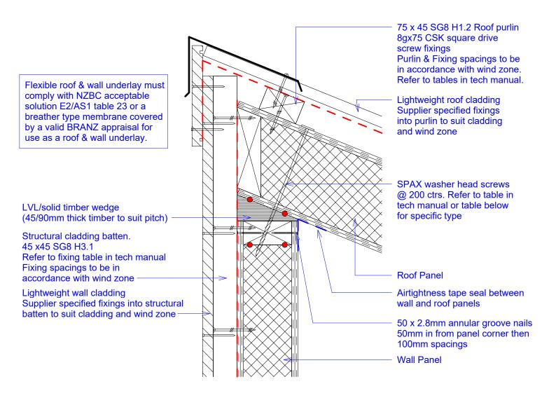
Washer Head type screws for fixing roof panels, wall panels and beams together are selected from the following.
