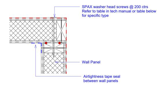
Washer Head type screws for fixing roof panels, wall panels and beams together are selected from the following.
