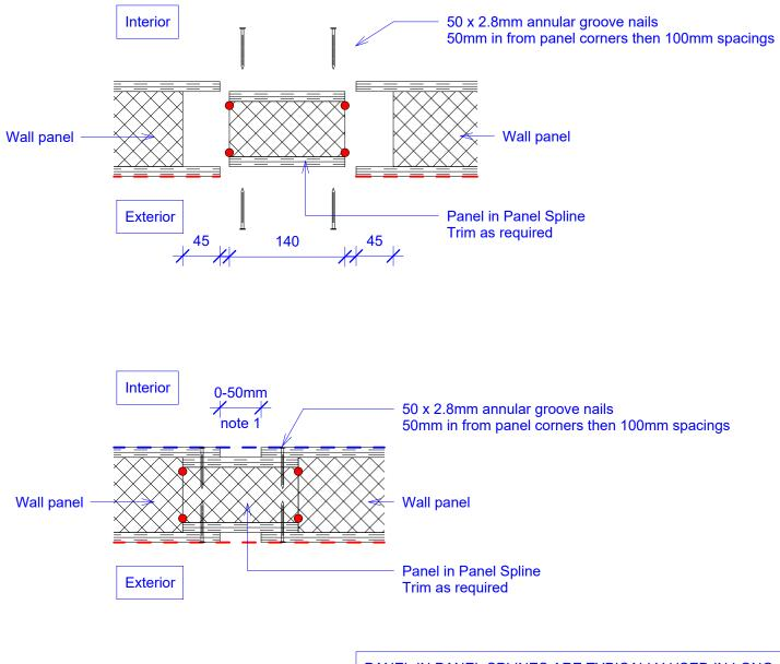
PANEL IN PANEL SPLINES ARE TYPICALLY USED IN LONG RUNS OF WALL PANELS TO INTRODUCE TOLERANCE Panel plan will set wall panels 25mm apart. Gap can be adjusted from 0-50mm
